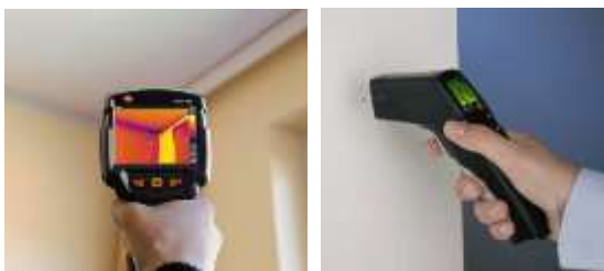
Figure 6. (Left) Thermal camera (Testo 865), (right) Infrared thermometer (Testo 830-T2)
