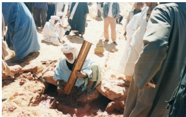
Figure 4. Operation of measurement using chekfa (photography Benziada, 2006).
