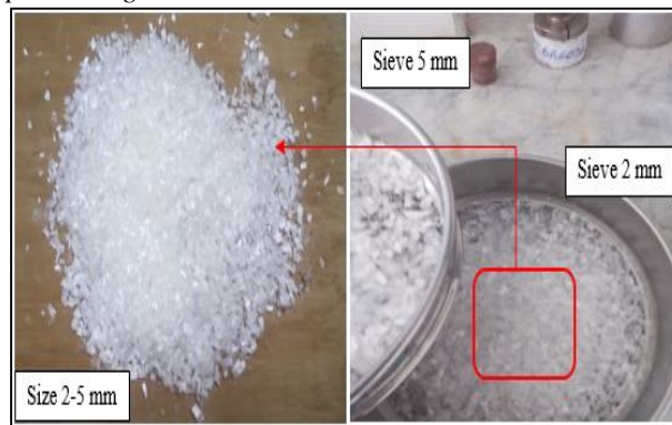
Figure 03. Shredded waste plastic bag of average size 2-5 mm
