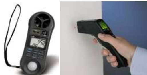
Figure 1. (left) Measurement instrument: a Thermo-Hygro -meter, (right) Infrared thermometer (Testo 830-T2)
