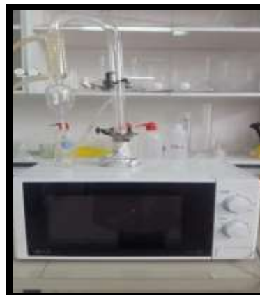
Figure 2. Hydrodistillation by microwave Clevenger distillation
