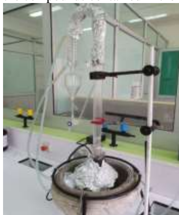
Figure 1. Hydrodistillation by Clevenger distillation apparatus.
