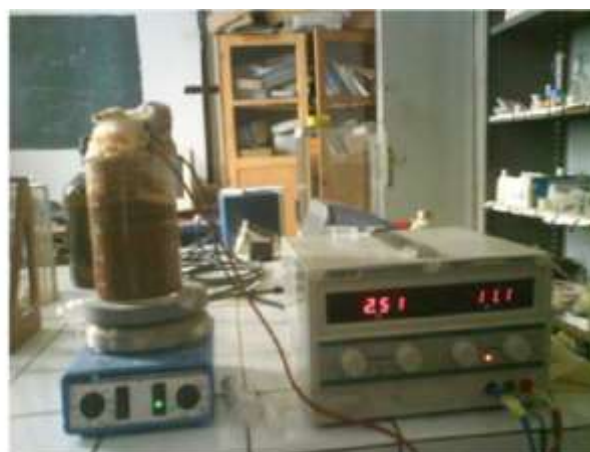
Figure 1. The electrochemical reactor in the laboratory experiments. (1) Beaker, (2) filter, (3) electrodes, (4) magnetic bar-stirrer, (5) magnetic stirrer, (6) DC power supply, (7) electric wire.
