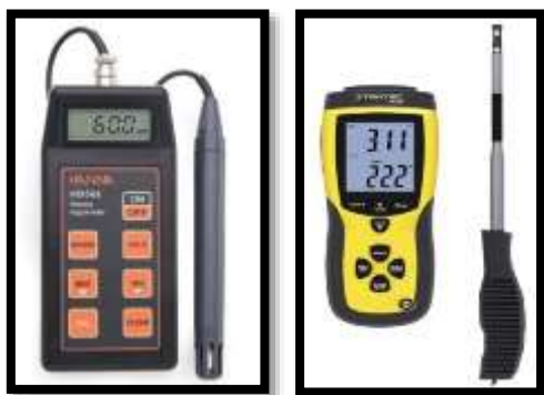
Figure 2. Measuring instruments, left thermal hygrometer [12], and right thermo-anemometer [13].
