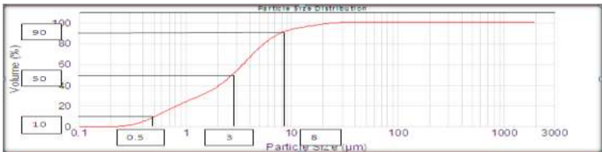
Figure 8. Particle size distribution of fly ash after grinding and sieving at 80 µm
