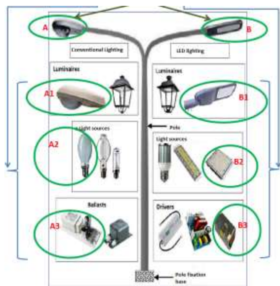
Figure 1. Components considered in the LCA comparative study in the case of a conventional street light pole (HPS) and one with LED
