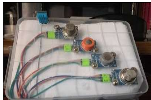
Figure 6. Positioning of the sensors in the holder
