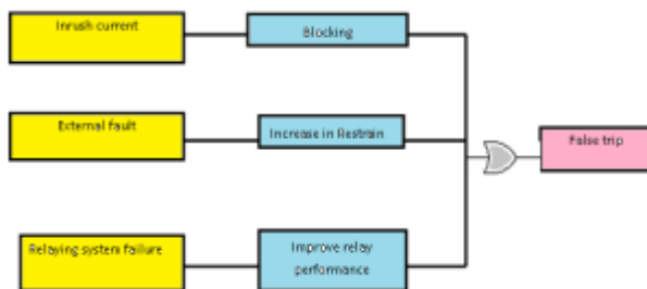
Figure 5. Root Cause Analysis (FTA) of unnecessary trip after providing mitigations
