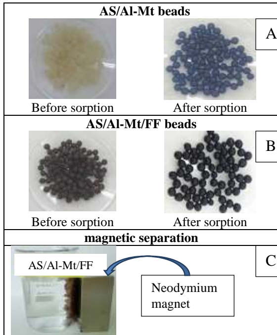
Figure 7. Photographies of the prepared biocomposite gelled beads, (A) before and after MG sorption on AS/Al-Mt beads, (B) before and after MG sorption on AS/Al-Mt/FF beads, (C) magnetic separation.
