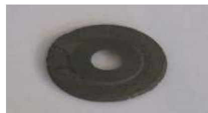
Figure 2. Image of a corroded Coupon Disc
