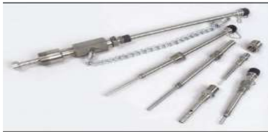
Figure 3. Electrical resistance probe ( ER)
