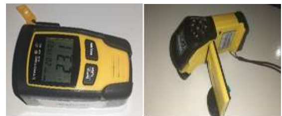
c. Temperature and humidity data Logger d. Thermal Imaging Camera
